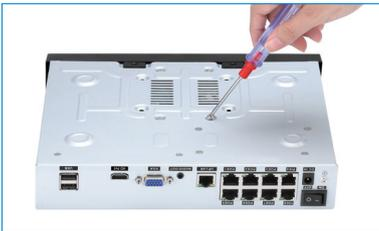
③ Screw HDD to the bottom
