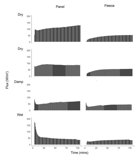
Figure 4. Heat fluxes recorded during the bench testing.
