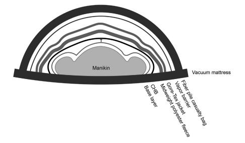
Figure 1. Experimental setup for hypothermia wrap. T indicates the temperature sensor position; CHB, chemical heat blanket.
