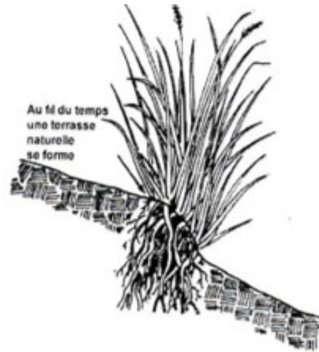
An illustration in the lesson showing how a Vetiver row holds the soil.
