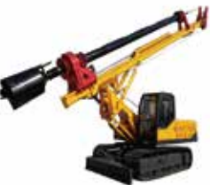
Rotary Drilling Rig
