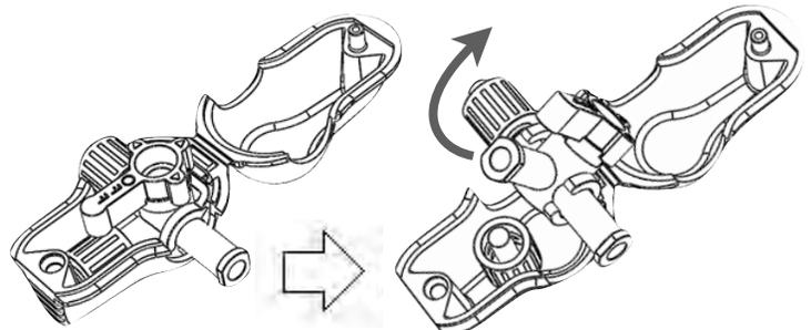
Figure 7. Accessing the Three-Way Stopcock.
