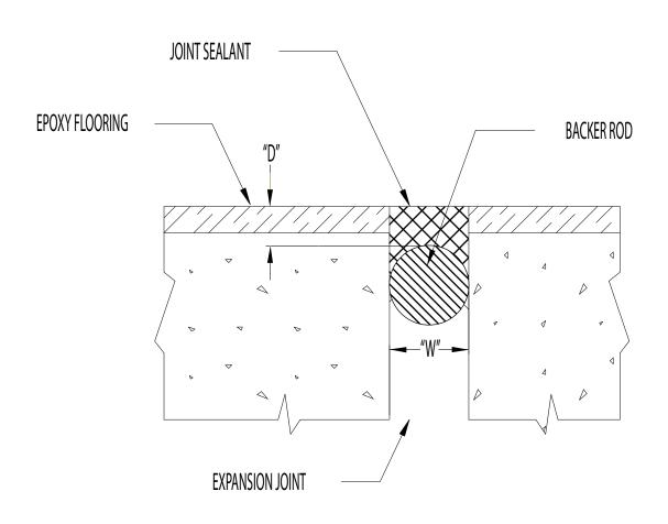
D = W/2 D = DEPTH OF BACKER ROD W = WIDTH OF EXPANSION JOINT
