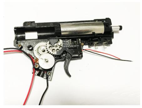
19. Clean the gearbox and gears, and use less gear oil as far as possible, so as not to pollute the sensors and affect the normal operation of DTU. After confirming that there is no problem, install the other side of gearbox and tighten the screws.
