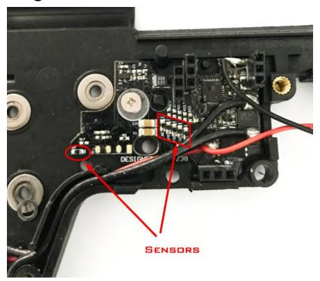
15. Make sure the other side of the gearbox is compatible with the DTU top board, if not modify it.
