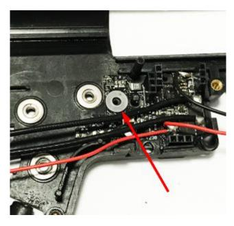
12. Secure the bottom board with cut-off lever screw. Make sure that the bottom board is not loose, otherwise it will affect the detection of the gear sensors.
