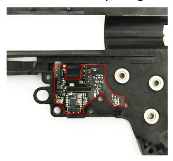
17. Put everything back into the gearbox, except 3 parts in step 8. Make sure the trigger does not touch the DTU.
