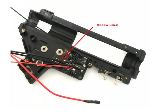
If there is a compatibility problem, it is recommended to modify the gearbox first, so that the bottom board can be installed into the gearbox smoothly.
