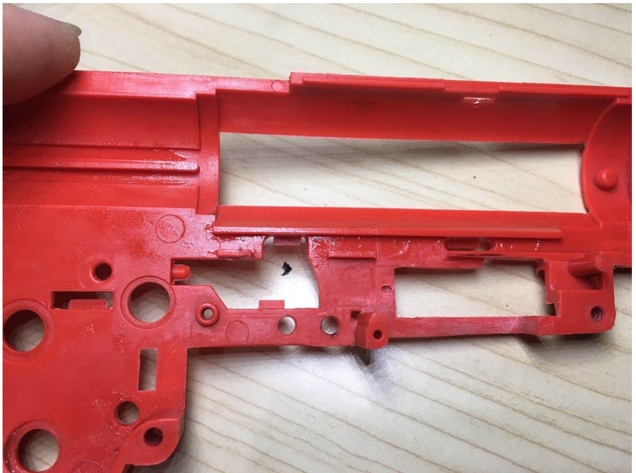
⑦ In addition, the maximum angle of rotation of trigger is not enough to reach the trigger sensor for AKA gearbox.
