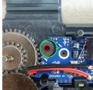
1. The green circle indicates the detection position of DTU gear sensors, and the red circle indicates the rotation axis
