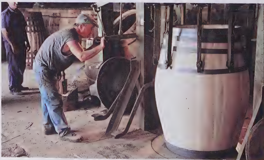
Finishing the cask by smoothing it down and ensuring it is tightly sealed. Cask assembly is a work of pure craftsmanship.
