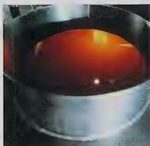
The product of mashing, the hot, malty, sugary liquid known as the worts, is drawn off ready for fermentation.
