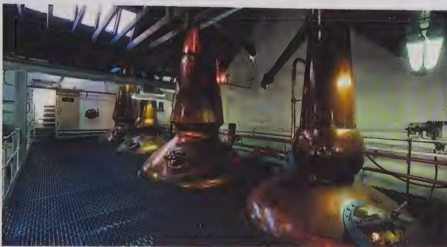
Boil-ball and lantern stills at Cragganmore Distillery. The 'boil ball' chamber at the base of the still-head (seen on the first still) causes heavier vapours to collect and fall back into the still to be redistilled.
