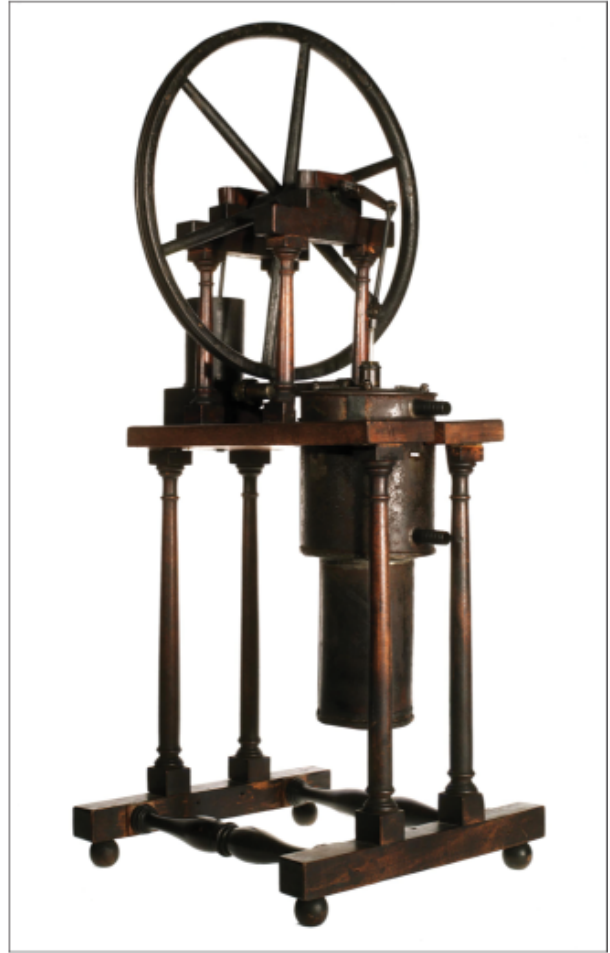
Plates 4 and 5. The Edinburgh Engine and the Glasgow Engine. Both were devised and built by young Stirling, presumably with help from the staff of the universities of the two cities, to which he appears at some point to have given the models. © National Museums Scotland, © The Hunterian, University of Glasgow)
