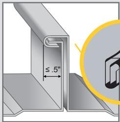
For horizontal seams under .5", crimp the seam to 180 degrees at desired clamp location.
