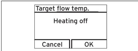
1. To switch off heating mode without switching off the hot water generation, press
