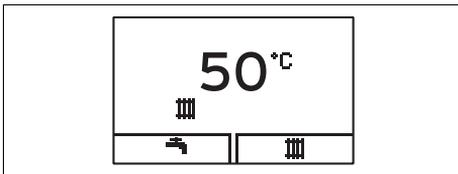
The basic display shows the current condition of the product. If you press a selection button, the activated function is displayed in the display.
