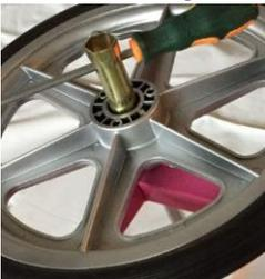
**STEP 6:** Insert a screw driver through the hole on **tool (I)** and twist to tighten. If the wheels do not spin, loosen the bolts slightly. See *Fig. 2*.
