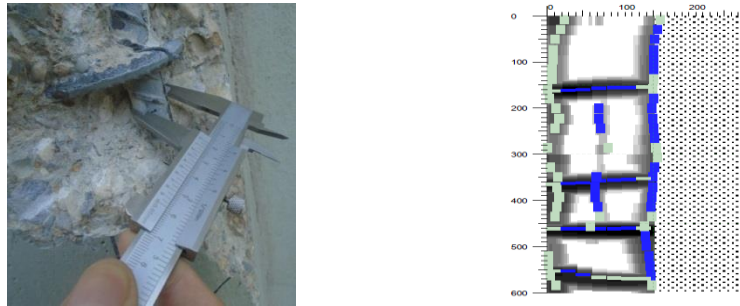
Figure 3. Identification of column reinforcement with clearing the cover and ferro-scan.
