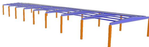
Figure 5: SAP2000 Structural Model
