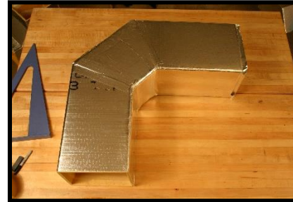
Diagonal cuts on LONG Horizontal Elbow
