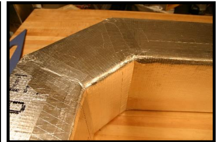
Diagonal cuts on SHORT side of duct
