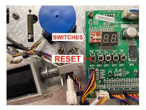
It is important that you only move the '4' position switch and not the '2' position switch when present.
