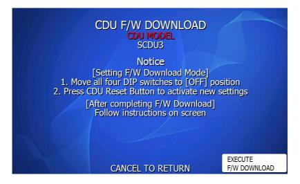
Follow the steps on the screen and move all 4 switches to the 'Down' position. Press the Reset button once you've done that.
