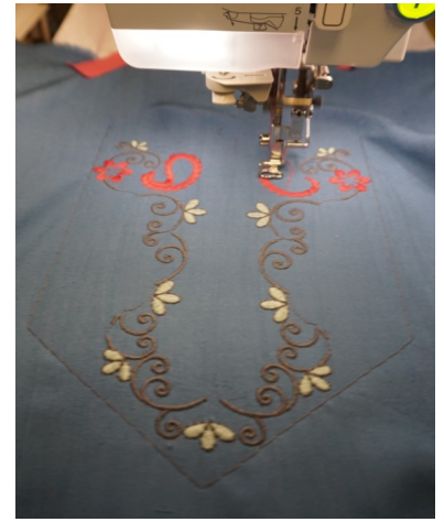
Line up center and marked neck with placement line and embroidery. Remove hoop do not take fabric off.
