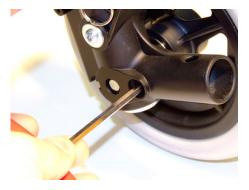
The pressure of the drag brakes on the hub and thus the rolling speed of the tires can be varied by loosening or tightening the interior set screws.
