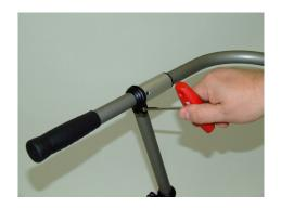
**FLUX size 1-3**: The depth of the grab rail must be set so that the anterior edge of the grip or the lower arm support pads on the grab rail lies behind the caster forks by at least the length of **A**. If bumper wheels are used the measurement of **A** must be increased with one centimetre. It is best to check this by placing the castor forks of the FLUX against a smooth door and measuring the space from the door leaf to the grip, i.e. forearm pad.
