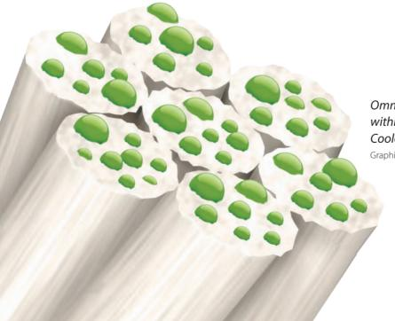
Omnitherm microcapsules within the threads of the Coolover fabric Graphic representation
