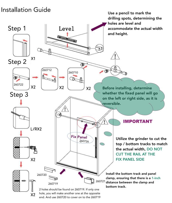
How to drill the hole on 260719? <u>Measure the width of the stationary panel plus 1 inch for the first hole, and mark it.</u> Then, mark the second hole 2 inches inward from the opposite end. Once drilled, mark and drill corresponding holes on the threshold. Securely attach the bottom track to the threshold with screws.
