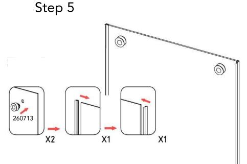
\* Install the two main wheels on the movable panel and attach the towel bar separately onto the fixed panel. Carefully handle and hang the panel onto the wall clip, ensuring caution is taken throughout the process. Check the alignment on the door edge and make any necessary adjustments to the positioning of the two main wheels for optimal functionality.
