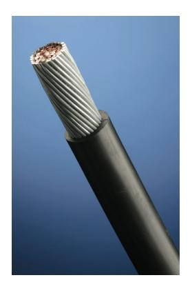
Theft deterrent composite cables are bare or insulated concentric stranded conductors that consist of peripheral galvanized steel stranding, which protects and conceals the internal tinned copper strands.
