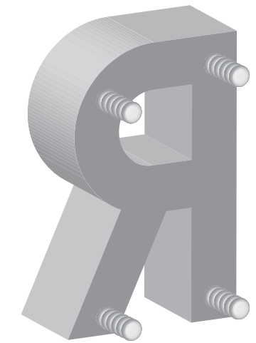
Stud Mounting - As Priced Requires minimum 1/4" thickness & 3/16" stroke.
