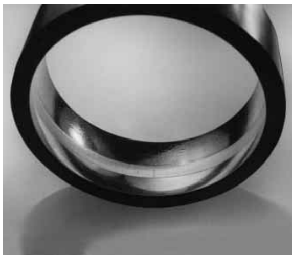
Cause of Failure: Loss of lubrication or the lack of lubrication (same idea, same outcome)
