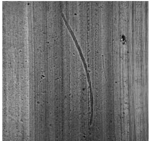
Cause of Failure: Dirt ingress during the lubricating process, seal damage, or bad installation practices
