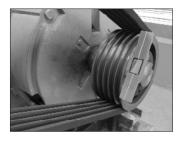
Using EZ Align<sup>°</sup> laser alignment tool showing laser line on target
