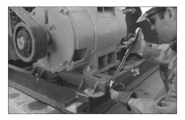
4. Move the motor in until the belt is slack and can be removed easily without prying. Never pry off a belt, as the sheave or sprocket can be damaged. Prying off belts also adds the risk of injury.
