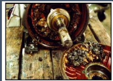
Motor that was Over-Lubricated
