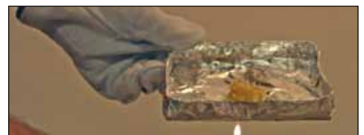
Fig. 77. A crackle test determines the presence of water in grease.
