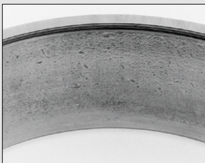
Fig. 9. Debris from other fatigued parts, inadequate sealing or poor maintenance caused bruising on this tapered roller bearing race.
