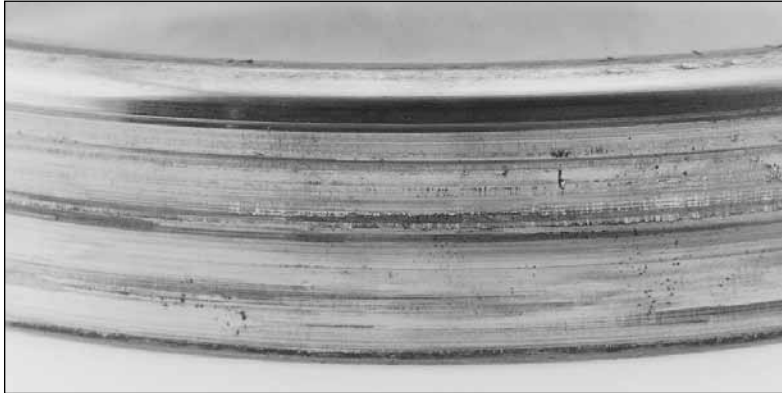
Fig. 49. A loose cup fit in a rotating wheel hub (typically tight) caused this bearing race damage.
