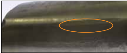
Fig. 67. This cylindrical roller flattened as a result of skidding
