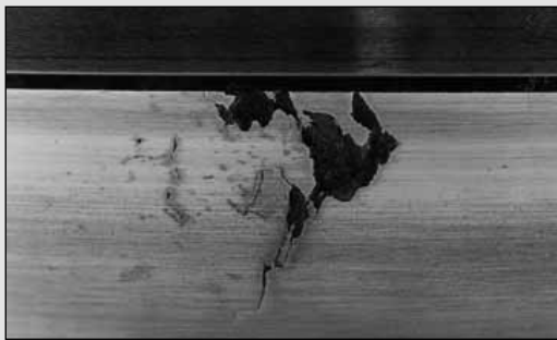
Fig. 23. PSO spalling resulted from debris or raised metal exceeding the lubricant film thickness on this tapered roller bearing inner ring.
