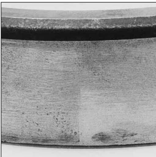
Fig. 47. The marks on the outside diameter of this cup are caused by a high spot on the housing. The cup race is spalled at the spot that corresponds to the spot on the outside of the cup marked from heavy contact.
