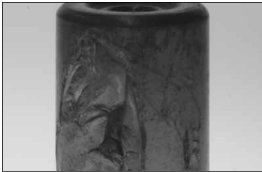
Fig. 27. Overloading on this cylindrical roller bearing caused roller surfaces to fracture.
