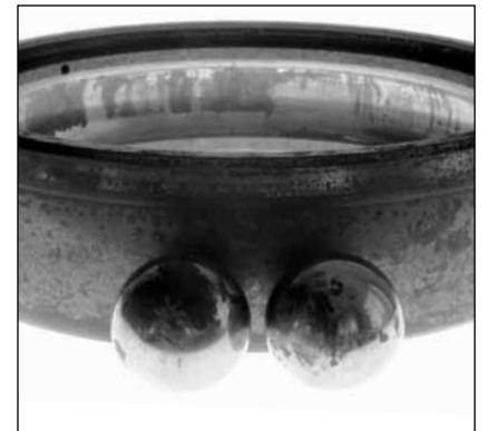
Fig. 15. This ball bearing outer race also depicts etching and corrosion.
