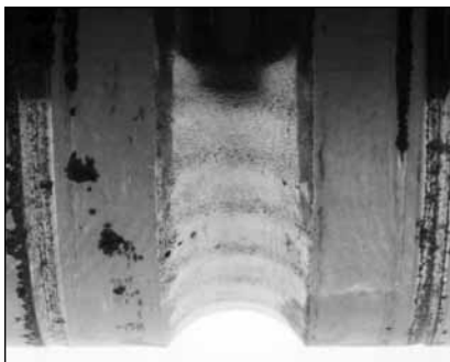
Fig. 56. Shock loading caused brinell damage on this ball bearing inner ring.
