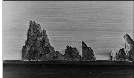
Fig. 22. Misalignment, deflections or heavy loading on this tapered roller bearing caused GSC spalling.
