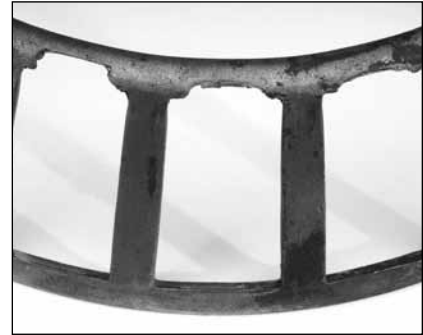
Fig. 33. Heavy wear in the small end of the cage pockets is typical of excessive endplay.
