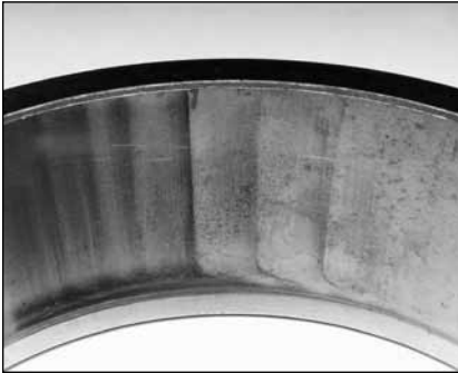
Fig. 31. Scalloping marks in the cup race are common with excessive endplay. Unloaded rollers enter the small load zone and are suddenly exposed to heavy loads.
