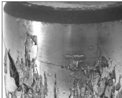
Fig. 24. Heavy spalling and fracturing from high loads on this spherical roller bearing.
