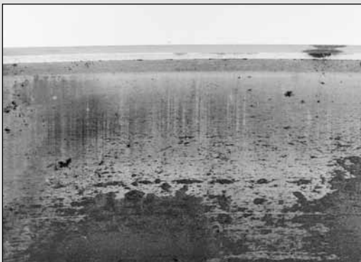
Fig. 17. Level 2 – Micro-spalling or peeling was the result of thin lubricant film from high loads/low RPM or elevated temperatures.
