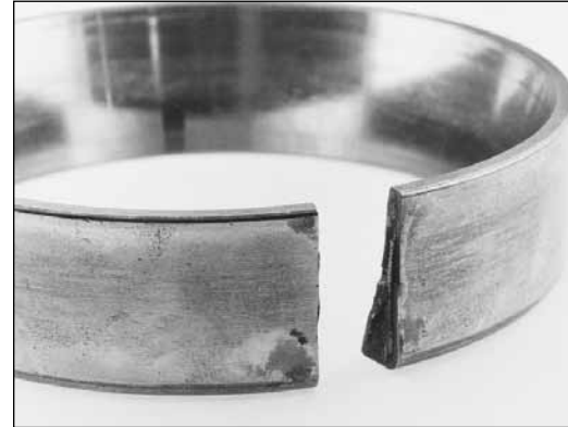
Fig. 50. This is what happens to a cup that is loose in a wheel hub. The cup turns and wears the cup seat so the fit becomes more loose. Then the cup starts to stretch or roll out. The cup, as it rolls out, continues to wear the cup seat and the cup continues to stretch. This process continues to the point where the stretch of the metal reaches the breaking point and the cup cracks open, as it has in this case.
