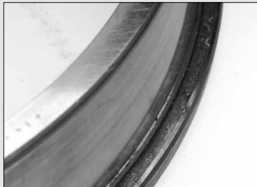
Fig. 18. Level 2 – Advanced rib scoring due to inadequate lube film.
