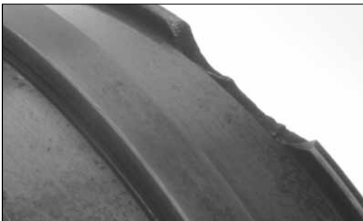
Fig. 39. This spherical roller bearing inner race depicts a fractured small rib caused by the use of improper installation tools.
