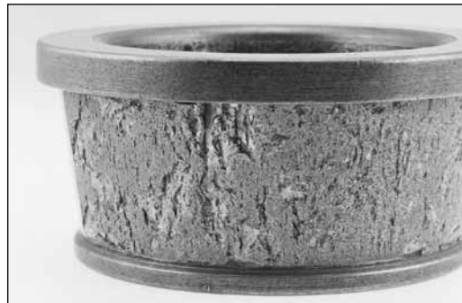
Fig. 28. High loads and low speeds caused insufficient lubricant film on this tapered roller bearing cone.
