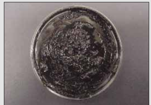
Fig. 64. This petri dish above contains heavily oxidized grease, which purged from an overfilled bearing. Grease undergoing heavy oxidation often has a very distinguishable black color and burned odor. In addition, it gets stiffer in consistency.
