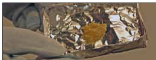
Fig. 76. To perform a crackle test, first put the grease sample on a piece of aluminum foil.
