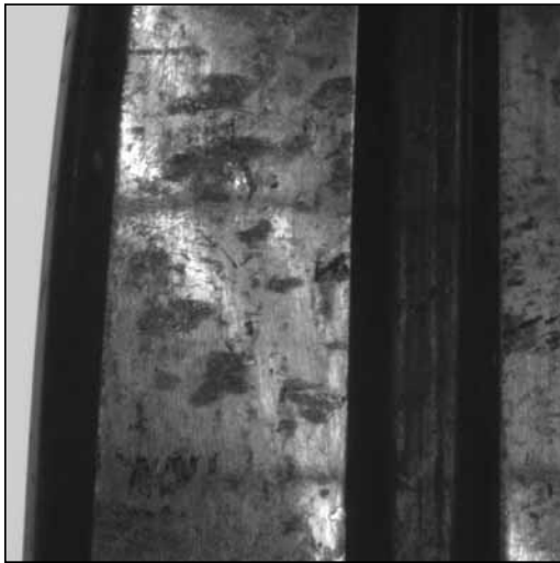
Fig. 45. A worn-out housing caused this bearing to lose fit and fret (move) during service. As a result, metal tearing and wear on this spherical outer ring occurred.
