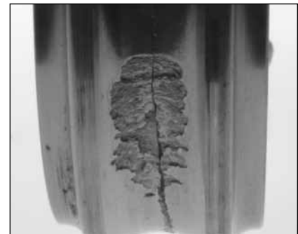
Fig. 26. This ball bearing inner ring depicts fatigue spalling from high loads. The fracture is a secondary damage mode.
