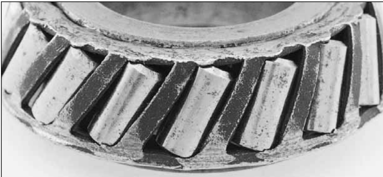
Fig. 43. Binding and skewing of these tapered rollers was due to the compression of the cage ring during installation or interference during service.
