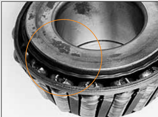
Fig. 20. Level 4 – Excessive heat generation caused advanced metal flow of the rollers, as well as cone rib deformation and cage expansion.
