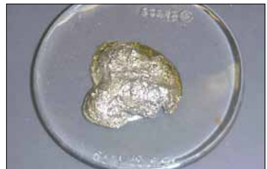
Fig. 66. Grease removed from an underfilled bearing shows shiny bearing metal debris.
