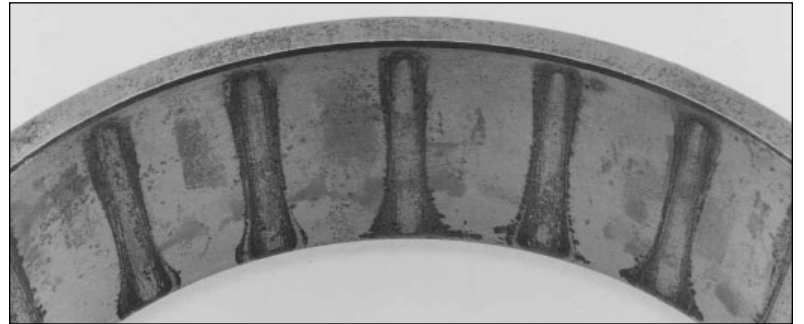
Fig. 12. This cup has heavy corrosion on the race. This type of corrosion may only be a surface stain without pitting. If the staining can be cleaned with a fine emery cloth or crocus cloth, the bearing may be reused. If there are pits that cannot be cleaned with light polishing, the bearing should either be discarded or, if practical, refurbished.
