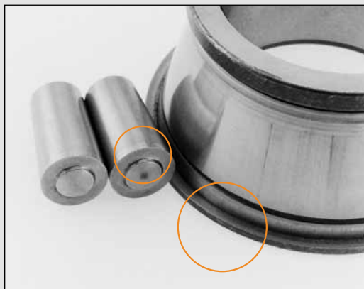
Fig. 1. Fine particle contamination entered this spherical roller bearing and generated wear between the cage surfaces, rollers and races.
