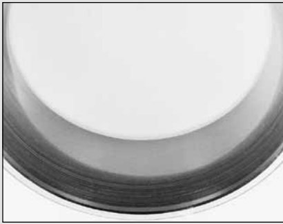
Fig. 35. Deflection, inaccurate machining or wear of bearing seats caused an irregular roller path on this tapered roller bearing outer ring.
