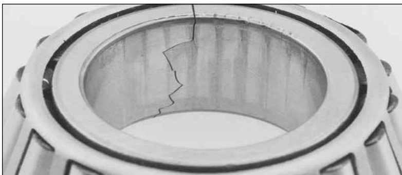
Fig. 52. An out-of-round or oversized shaft caused this fracture on a tapered roller bearing cone.
