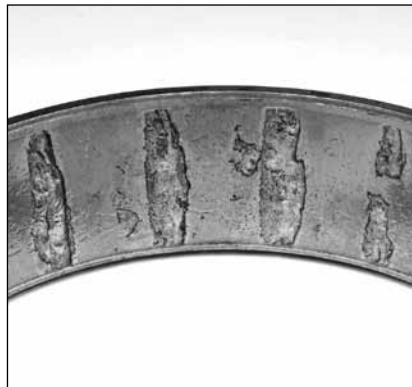
Fig. 13. Advanced spalling initiated at water etch marks on the cup race makes this bearing unsuitable for further service.
