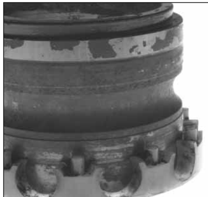
Fig. 14. Heavy water damage is shown on this ball bearing inner ring and cage.
