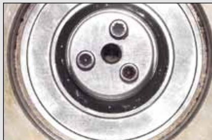
Fig. 65. 'Clean' grease slightly purging (leaking) from a bearing during initial start-up is generally acceptable. The grease is wet and evenly purged. If this slight purge is not causing any problems, leave it alone as it is an effective barrier seal.
