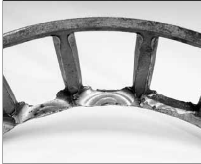
Fig. 32. Cage pocket damage from excessive roller movement.
