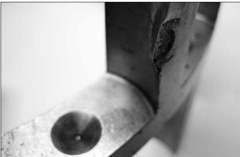
Fig. 44. Poor handling practices caused a deep dent on this spherical roller bearing cage bridge. This damage will result in a lack of proper roller rotation, possible roller skidding, increased temperatures and decreased life.
