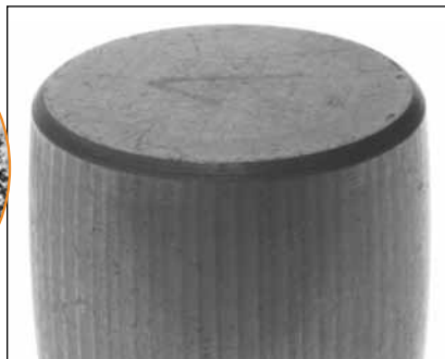
Fig. 60. Welding on a machine, while the bearings were rotating, caused electric arc fluting on this spherical roller bearing.
