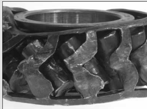
Fig. 21. Level 4 – Total bearing lockup is depicted here.
