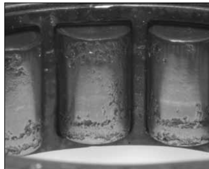
Fig. 25. High loads resulted in fatigue spalling on this cylindrical roller bearing.
