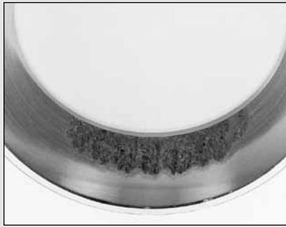
Fig. 36. This irregular roller path is 180 degrees opposite of Fig. 35.
