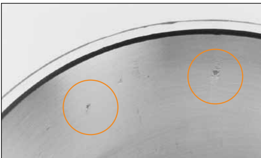
Fig. 41. Tapered roller spaced nicking was caused by the roller edges hitting the race during installation. These nicks/dents have raised edges that can lead to excessive noise, vibration or act as points of stress concentration.
