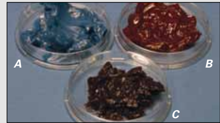
Fig. 69. Grease A and Grease B are not compatible. When mixed together they become lumpy, discolored and hard in composition (Grease C).
