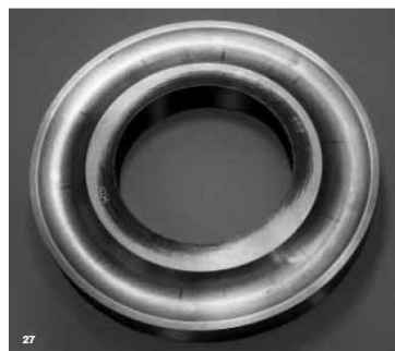
Fig 27 Washer of a thrust ball bearing subjected to overloading while not running. The indentations are narrow and radially aligned, not spheroid as in radial ball bearings.
