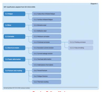
**Bearing Failure Modes**
