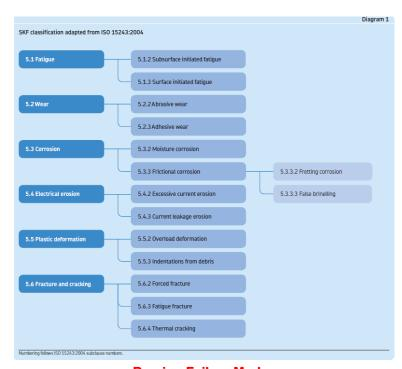
**Bearing Failure Modes**
