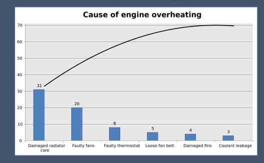
This technique helps to identify the top portion of causes that need to be addressed to resolve the majority of problems.
