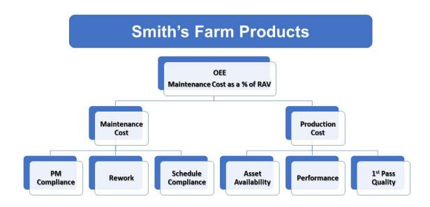
Leading indicators such as Percent of Rework and Percent of PMs Executed on Time (PM Compliance) affect the overall performance of the maintenance process (to include they impact the production process), which results in a certain level of performance.)
