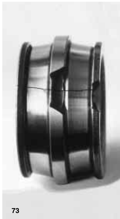
Fig 73 Cracked inner ring of a spherical roller bearing. One roller has been removed to allow the raceway of the left-hand of the photograph to be examined. The roller has then been hammered back in place, causing part of the centre flange to break away. The impacts have been transmitted via a roller in the other row and part of the outer flange has broken off too. At the same time the ring has cracked right through
