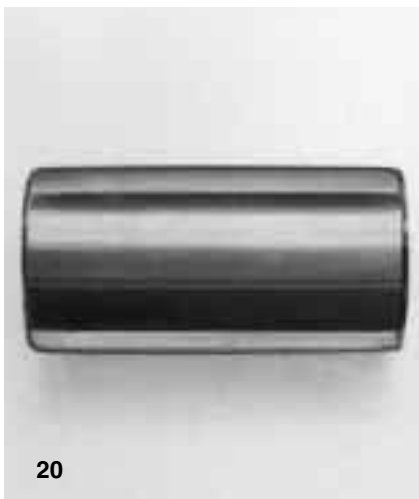
Fig 20 Cylindrical roller with mirror-like surface on account of lubricant starvation
