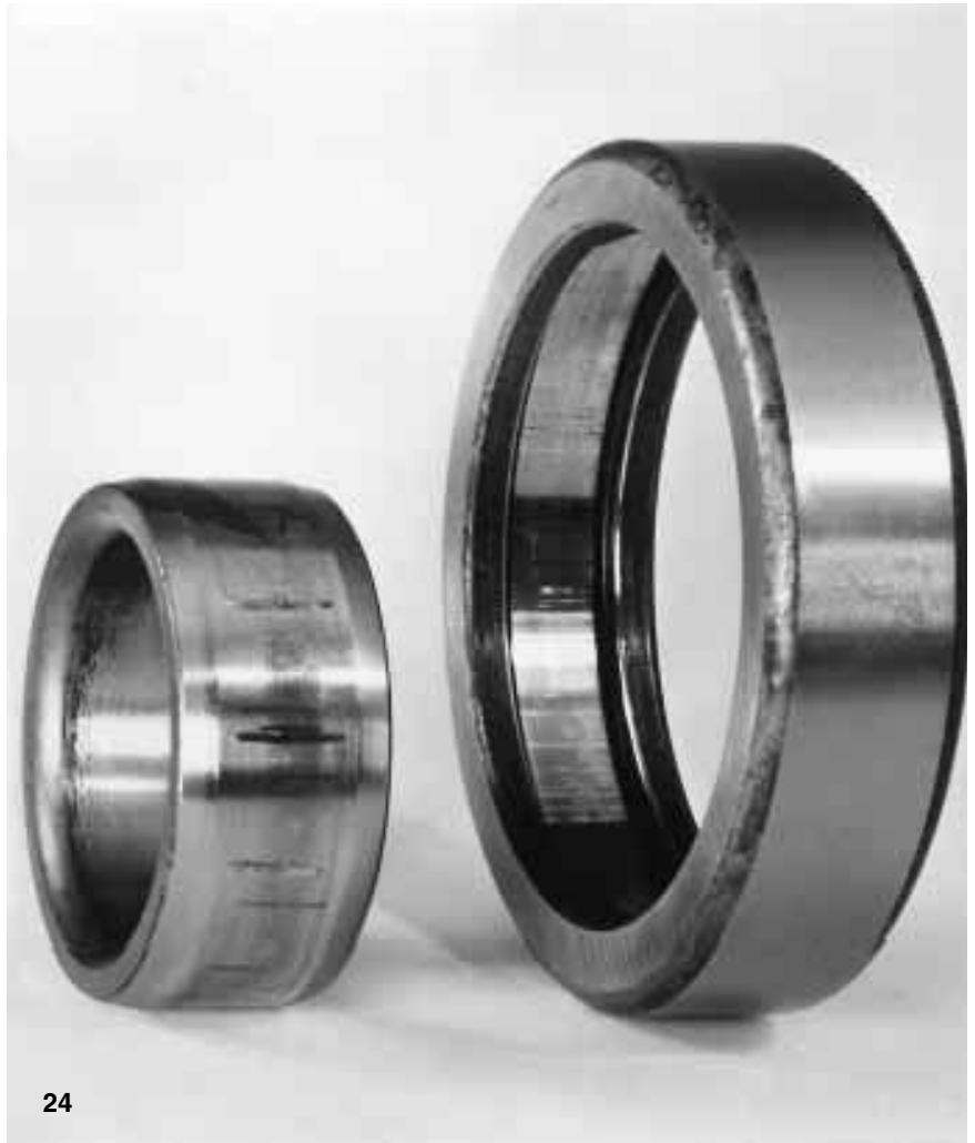
Fig 26 Outer ring of a self-aligning ball bearing damaged by vibration. The bearing has not rotated at all
