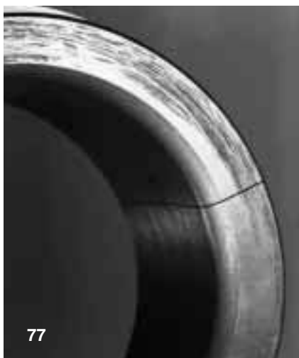
Fig 77 Spherical roller bearing inner ring that has cracked right across following smearing of one face. The ring has been mounted to about a spacer that has not had a sufficiently tight fit on the shaft. Consequently the spacer has rotated relative to the shaft and the bearing ring
