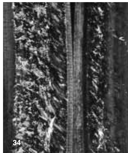
Fig 34 Guide flange smearing attributable to the same causes as the smearing shown in fig 33
