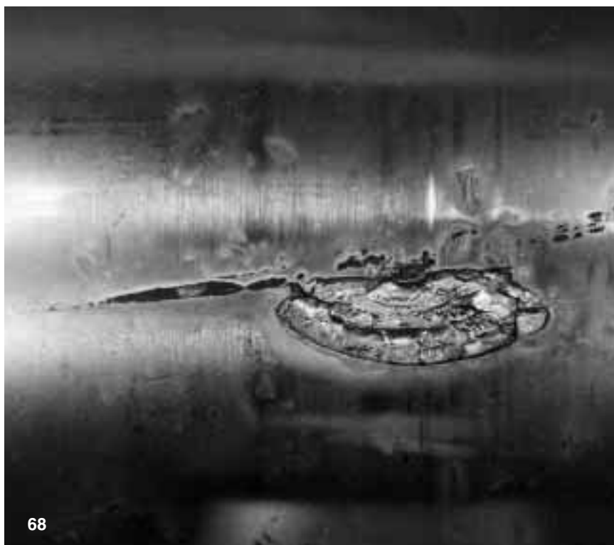
Fig 67 Cross section through the roller depicted in fig 66, showing the way in which the fatigue crack extends beneath the surface. The fully developed flaking originated in the same manner
