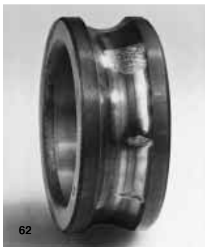
Fig 62 Various stages of flaking in the inner ring of a deep groove ball bearing. The ring has been mounted with interference fit on the shaft and blows have been directed against the outer ring, causing the mounting force to pass through the balls, which have produced the indentations
