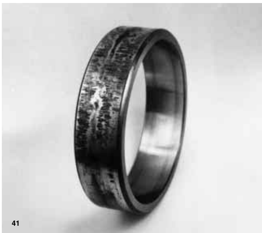
Fig 41 Smeared outside surface of a spherical roller bearing outer ring. Material transfer has occurred from housing bore to bearing ring
