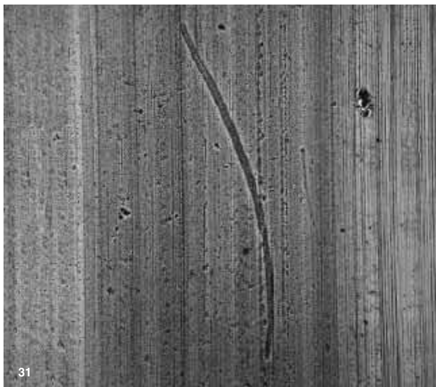
Fig 31 Indentations, caused by dirt, in one of the raceways of a roller bearing – 50 × magnification
