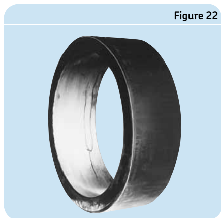
Cracks caused by faulty housing fit
