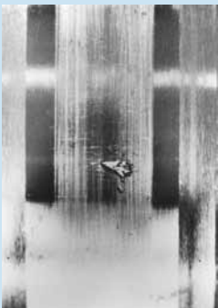
Early fatigue spalling
