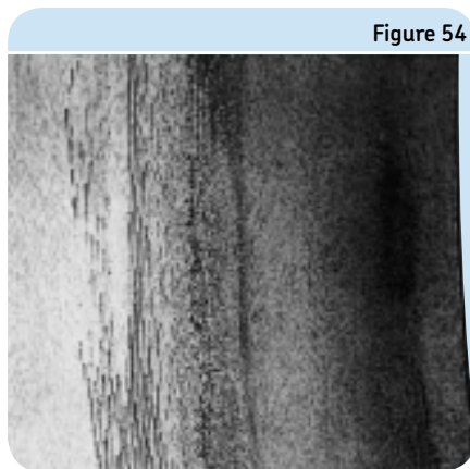
Corrosion streaks caused by water in the lubricant while the bearing rotated
