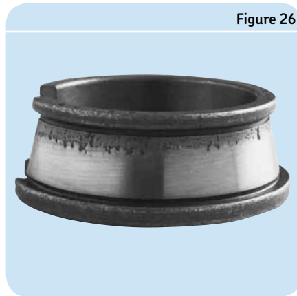
Fatigue caused by edge loading
