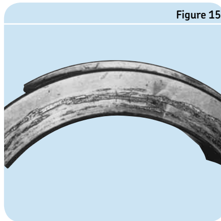
Smearing caused by contact with the shaft shoulder while bearing ring rotated
