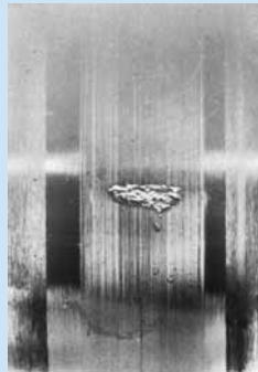
More advanced spalling
