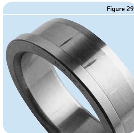
Smearing caused by excessive force in mounting
