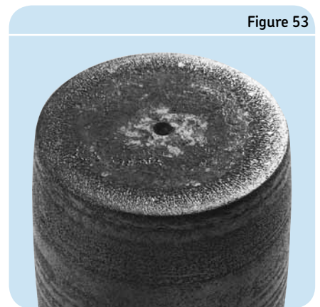
Rust on end of roller caused by moisture in lubricant
