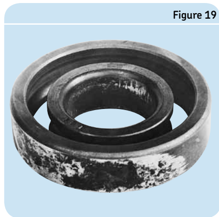
Wear due to fretting corrosion
