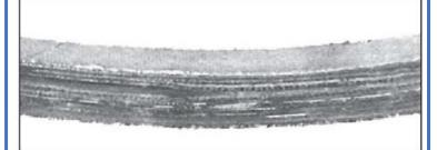
**Cause of Failure** — Constant slippage caused by insufficient tension in belt. **Correction** — Tension drive in accordance with the recommendations of the equipment manufacturer and this manual.
