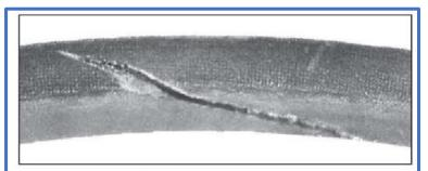
Cause of Failure — Cut bottom and sidewall indicate belt was pried over sheave and damaged during installation. Correction — Be sure to use proper length belt and move tensioning all the way "in" when installing belt.
