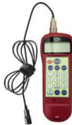
3. Another tool to use is simple tool to measure tension and deflection using a tension gauge.
