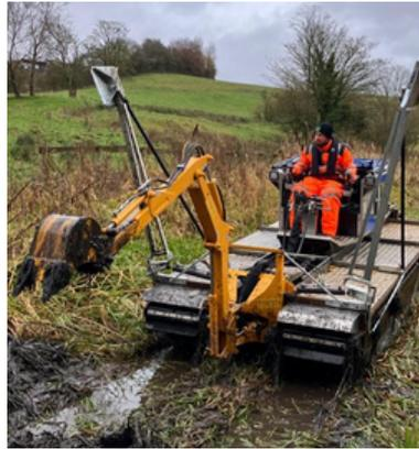
WE HAVE BEEN PROVIDING EFFECTIVE WATERWAY IMPROVEMENT SERVICES, INCLUDING THAT ON THIS ABANDONED CANAL IN MANCHESTER, PICTURED LEFT, WHERE WE UTILISED TWO OF OUR AMPHIBIOUS TRUXOR BOATS WITH DIGGER ARM ATTACHMENT TO CLEAR A CHANEL AND CREATE FREE FLOWING WATER.
