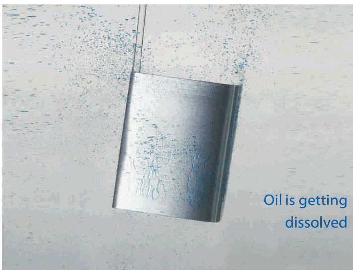
Emulsified oil drops are dissolved in the solution
