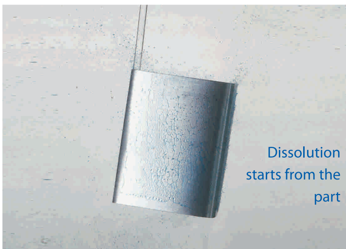
Short after dipping, removing starts
