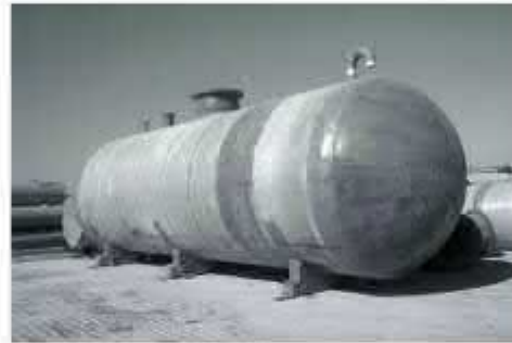
GRP/FRP Tank and Manholes
