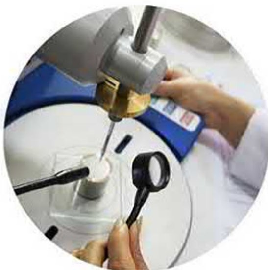
Paraffin Wax Consistency Test
