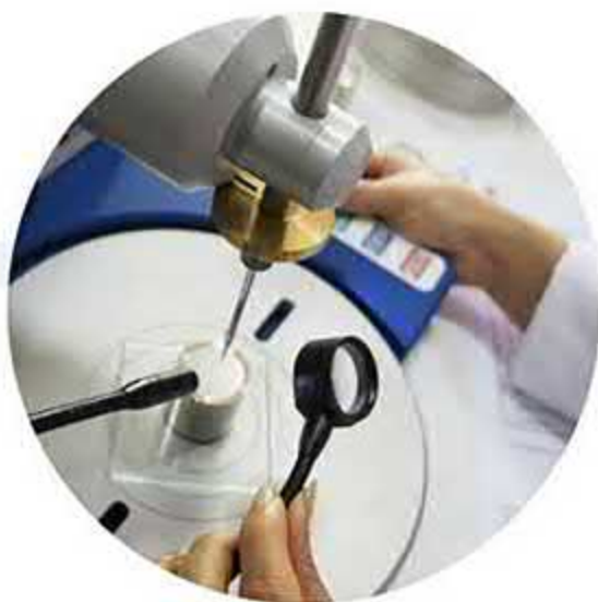
Paraffin Wax Consistency Test
