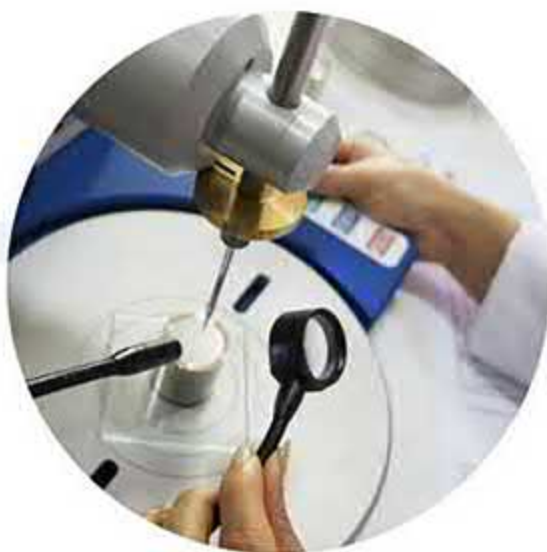
Paraffin Wax Consistency Test
