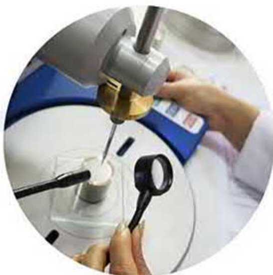
Paraffin Wax Consistency Test
