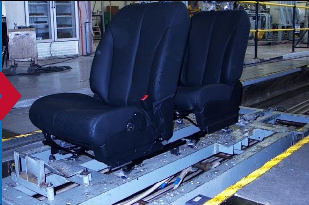
Seat (fixed to sliding structure) sliding forward/rearward into dead stop with 196 m/s<sup>2</sup> acceleration
