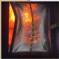
Top: Annealed Glass Filmed with SafetyShield 1500.
