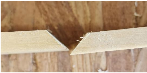
12: Miter to keep best side of the board on the outside
