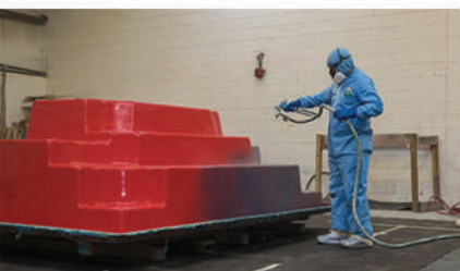
One of our premium Gelcoat colors is the first layer that is sprayed onto the mold to create your new pool.
