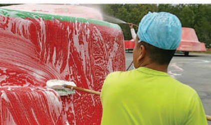
The mold is cleaned and prepared to build your pool on.
