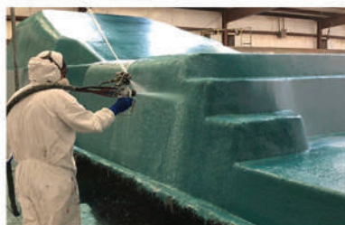
Vinyl Ester Resin, reinforced with chopped strand fiberglass, is applied after the gelcoat.
