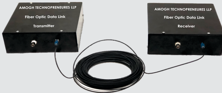
Transmitter and Receiver Connection with POF cable
