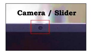
Most Laptops have a **Camera** built into the <u>top of the screen</u>. Make sure the cover (slider) is **Open**.
