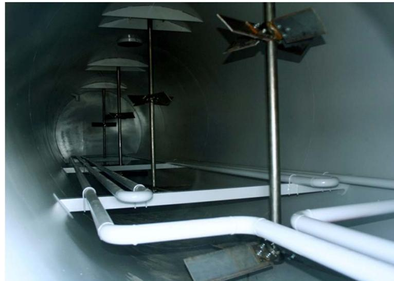
Steam & hot water traced systems for use primarily in the Bakken Shale or water reuse areas that require heating the fluid with chemicals for the break or increased polymer yield and gel strength.
