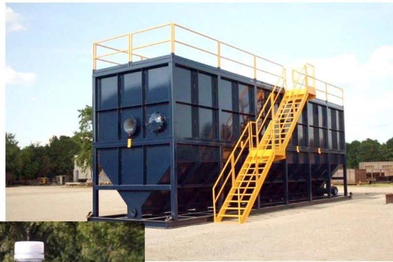
Specialty treatment equipment is being developed for water reuse. Currently cleaning pipeline pigging and frac tank waste in Louisiana with great success. The protocol for water reuse will be coming out in 2014.
