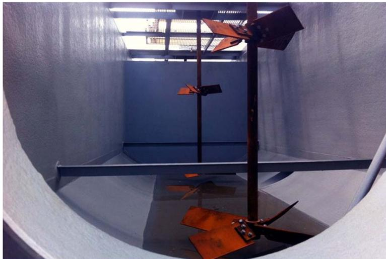
Specialty turbine agitators for biopolymeric gel development, emulsion polymer yield for water reuse – the flocculation of oil and solids ending in downstream filtration or belt pressing. There are multiple applications of these turbine tanks for drilling, workover, and completion operations.
