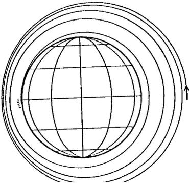
Circular Orbit Life  $\approx \frac{.15 \text{ m}^2 \text{ yr}}{\text{kg}} \frac{M}{C_D A} \frac{(1 + 2.9(r-6578)/\text{Tex})^{11}}{3000 - \text{Tex}}$
