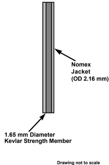
Fig. 9. A magnification of the baseline tether.
