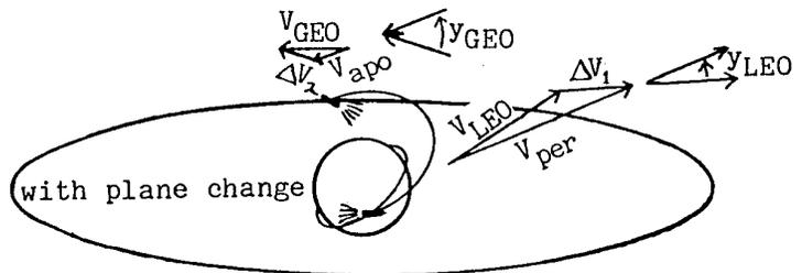
Total  $\Delta V$  is minimized when  $\frac{\sin \gamma_{LEO}}{\sin \gamma_{GEO}} = \frac{r_{LEO}}{r_{GEO}}$
