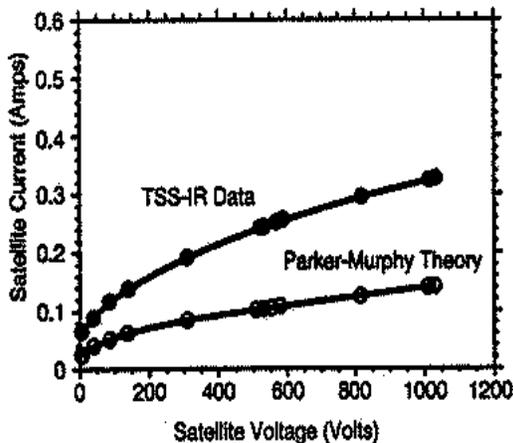
Figure 1.4 Measured TSS-1R and theoretically predicted I-V characteristics
