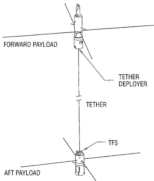
Figure 1.24 OEDIPUS-C configuration with location of the TFS
