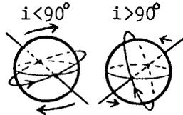
For sun-synchronous orbits: ( $i = 100^\circ \pm 4^\circ$ )
