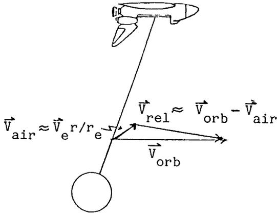
$$F_{drag} = .5 \int \rho C_D v_{rel}^2 \text{ Width } \delta r$$
