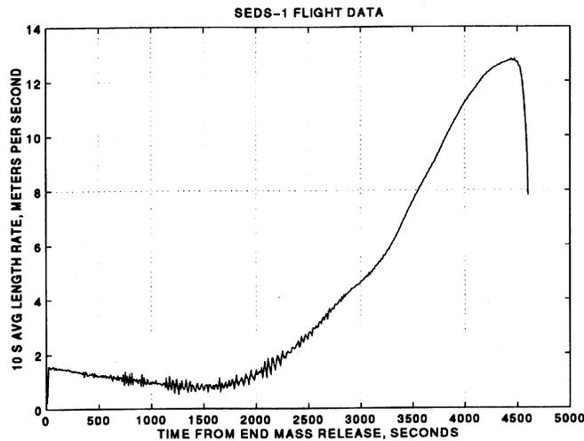
Figure 1.13c. SEDS Deployer 10-sec Average Length Rate
