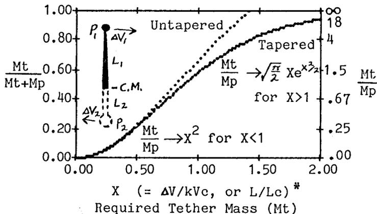
\*  $k = \begin{cases} 1.00 & \text{for spinning operations} \\ 1.15 & \text{for hanging} \\ 1.21 \pm .01 & \text{for swinging} \\ 1.41 & \text{for winching} \end{cases}$
