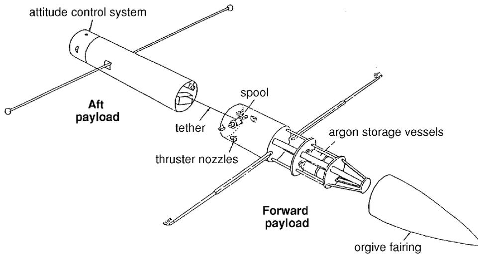
Figure 1.22 Some subsystems in the OEDIPUS-A payload configuration
