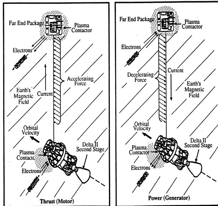
Figure 1.15 PMG investigation of an electrodynamic tether
