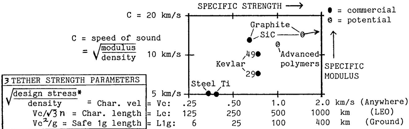
\* Design stress is assumed to be 1/2 the ultimate strength for metals and 1/4 the short-term individual fiber strength for other materials.
