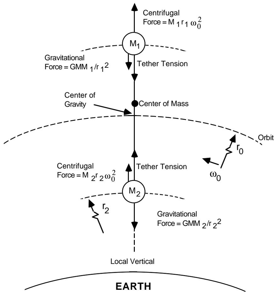
Figure 4.1 Forces on Tethered Satellites
