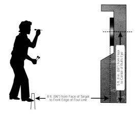
*Note:* Attention should be given that the measurement is from the "Foul Line" to the "Face" of the dart board and *not* from "Foul Line" to the front of the machine cabinet.
